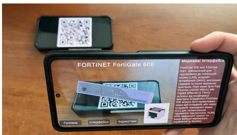
Figure 6 – AR app to study the structure and functionality of the FortiGate 60E firewall
